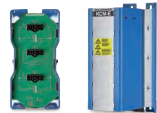
The energy reserves can increase almost unlimitedly with the expansion modules KCM-E. A discharge resistor is integrated into every module. The connection is made to connectors on the top side of the module using the cable protected against polarity reversal that is supplied.
