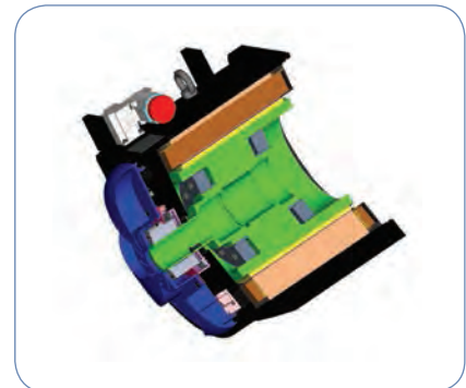
Design of a Cartridge DDR motor (CDDR)
